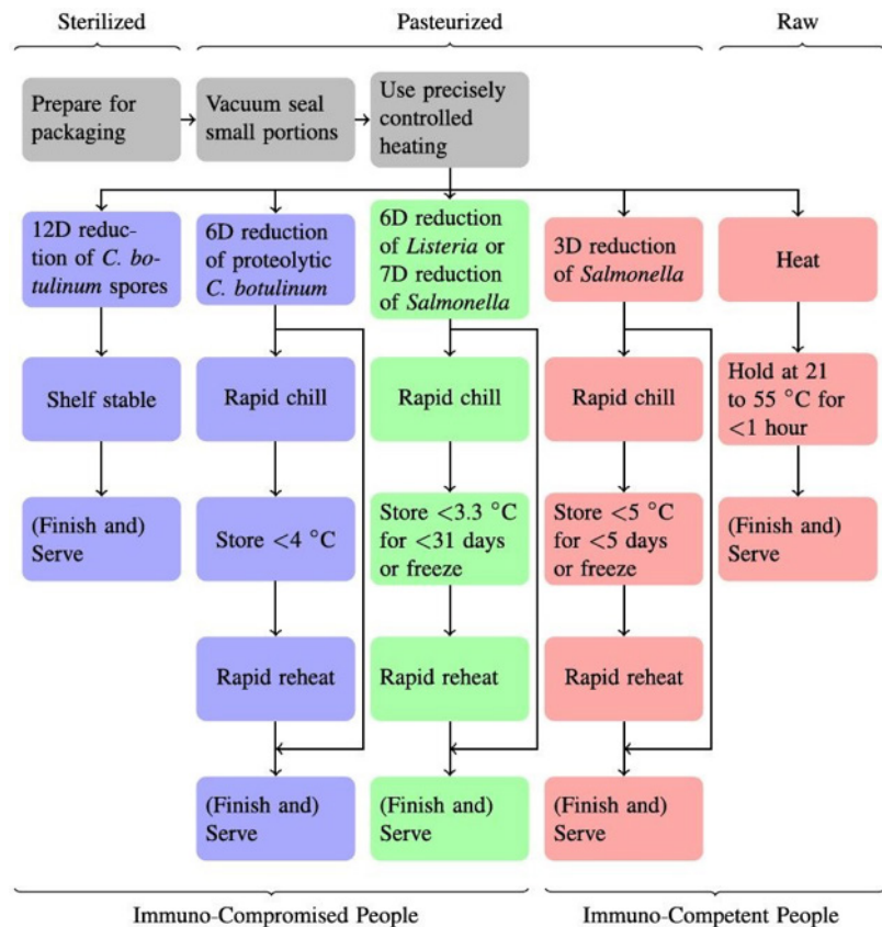
Fig. 1: Flow diagram, sous vide cooking. The branches in red and green (the rightmost three) are common in both restaurants and home kitchens while industrial food processors only use the branches in blue and green (the leftmost three). The branches in red (the rightmost two) should only be served to healthy immune-competent people and in the rightmost branch; they should understand and accept the risk. (Baldwin 2012).
